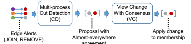
Figure 3: Solution overview, showing the sequence of steps at each process for a single configuration change.
