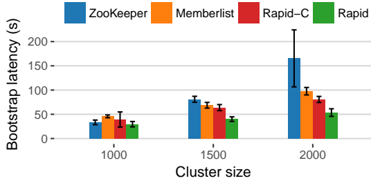
Figure 5: Bootstrap convergence measurements showing the time required for all nodes to report a cluster size of N . Rapid bootstraps a 2000 node cluster 2-2.32x faster than Memberlist, and 3.23-5.81x faster than ZooKeeper.
